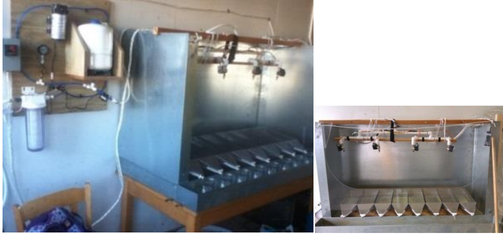
Figure 2 - Overhead leaching apparatus used to evaluate the effects of BMP procedures on migration of metals from ACZA, CA or ACQ treated wood.
