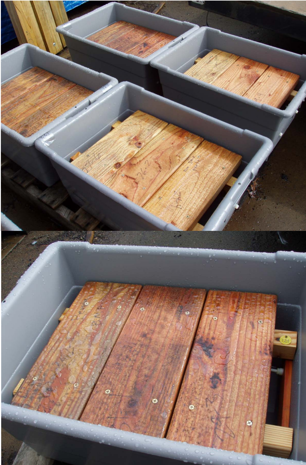
Figure 1 Examples of penta treated wood decks exposed to rainwater in Corvallis, OR.
