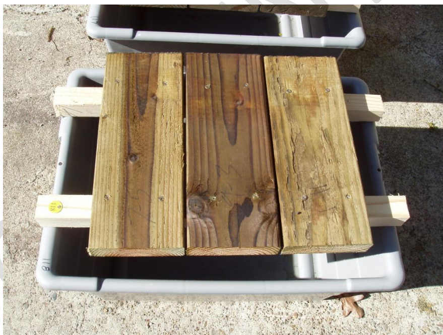
Figure 1 Examples of penta and copper naphthenate treated wood decks exposed to rainwater in Corvallis, OR in BMP Deck Trial 1.
