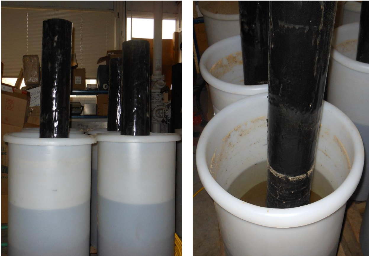
Figure 15. Example of a polyurea coated ACZA treated Douglas-fir piling.
