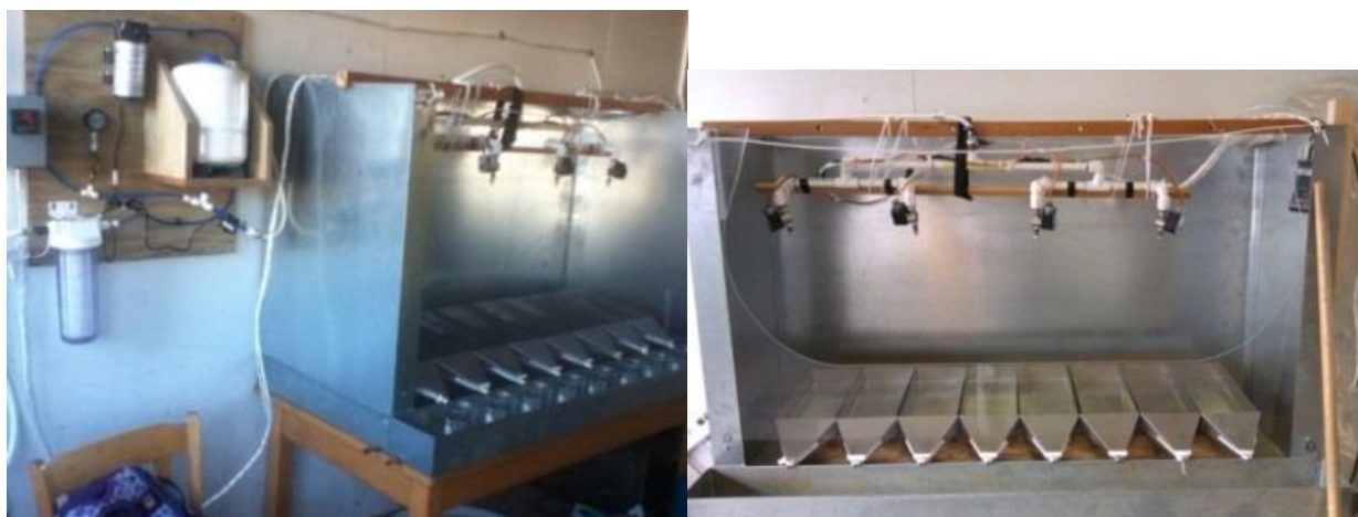
Figure 1 - Overhead leaching apparatus used to evaluate the effects of BMP procedures on migration of metals from ACZA, CA or ACQ treated wood.
