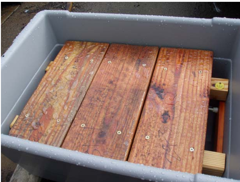
Figure 1 Examples of penta treated wood decks exposed to rain-water in Corvallis, OR.
