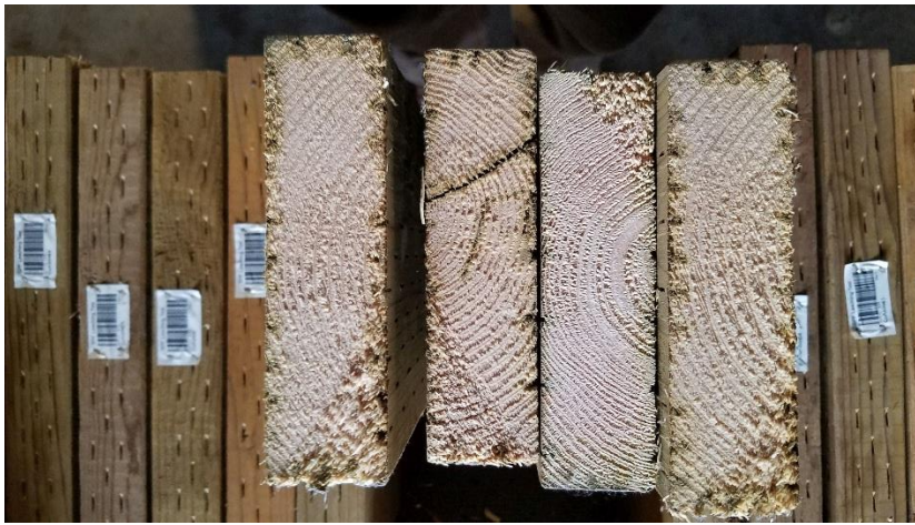
Figure 2. Photos showing poor preservative penetration in SPF boards treated with CCA (A), CA (B) or ACQ (C).
