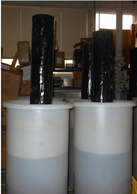
Figure 14. Example of polyurea coated piling in exposure tanks
