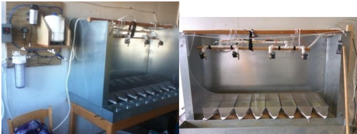
Figure 1 - Overhead leaching apparatus used to evaluate the effects of BMP procedures on migration of metals from ACZA, CA or ACQ treated wood.
