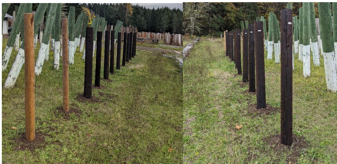
Figure 1.4.1: Photos of the creosote-treated Douglas-fir and southern pine posts at the Peavy Arboretum
