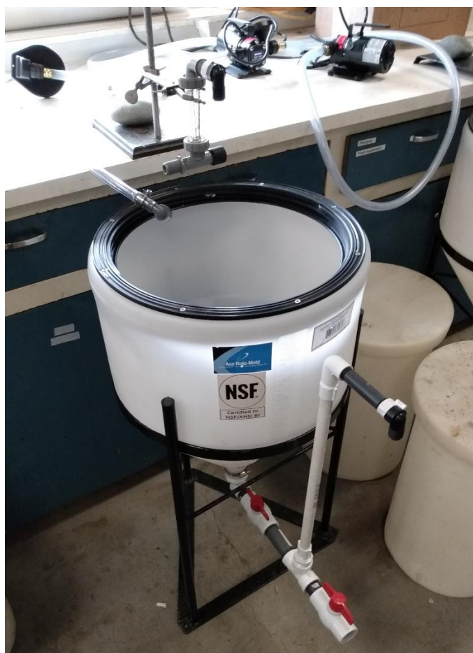
Figure 2.1.1: Commodity scale leaching apparatus made out of a cone-bottom tank with an overflow collection point with a flow meter above the tank.
