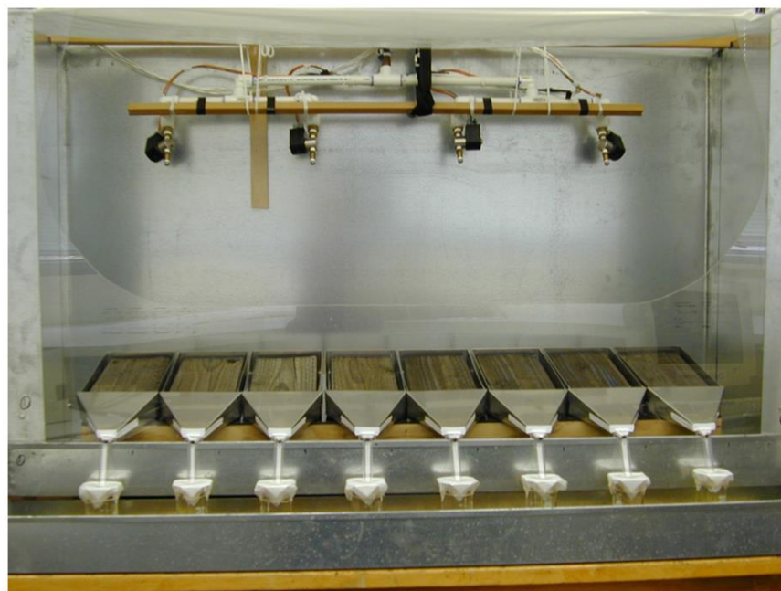
Figure 1.1.1 Overhead leaching apparatus used to evaluate the effects of BMPs on metal migration from preservative treated wood.
