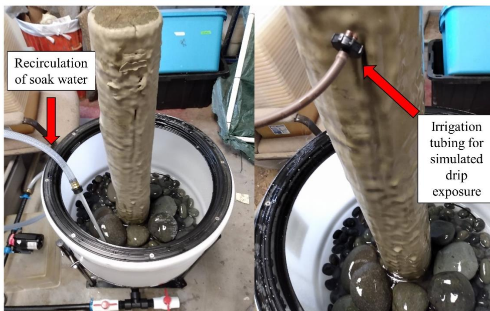
Figure 2.1.2: Demonstration of recirculation function of the prototype leaching apparatus (left) and drip leaching functionality (right). Further modifications will need to be made to run this apparatus in a test.
