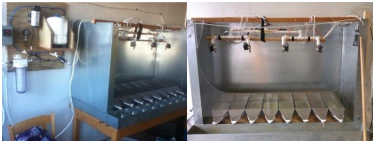
Figure 1. Overhead leaching apparatus used to evaluate the effects of BMPs on metal migration from preservative treated wood.
